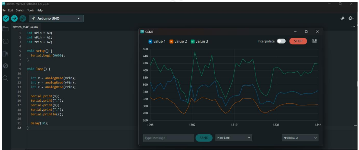
Fig.7: Serial plotter output — X, Y, Z axis acceleration values
