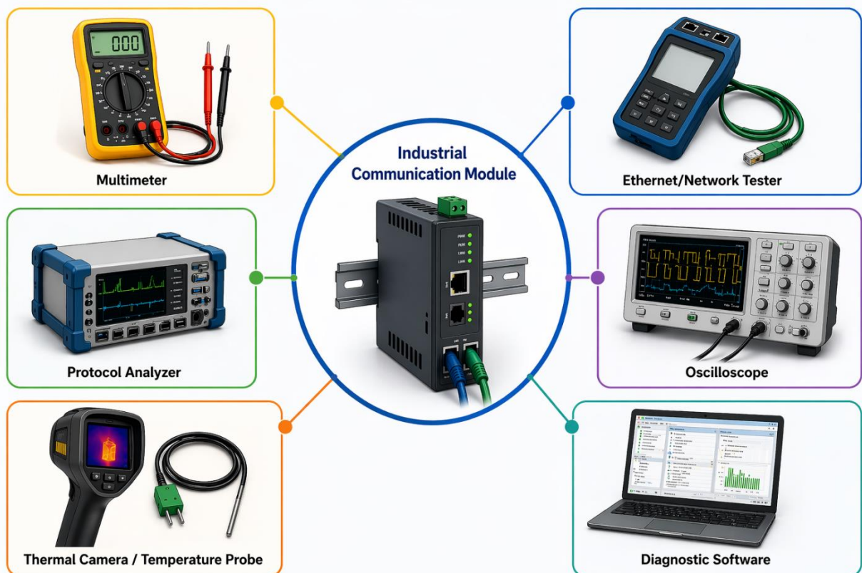
Fig.3.13: Tools Used for Communication Module Hardware Testing
